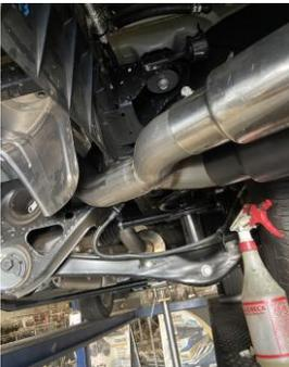
5. Finally, over axle pipe #C can be installed using the Band Clamp #D. Once the over axle pipe is in you may install Exit Pipe #E along with both Tips. (Tighten all clamps working from front to back.)
