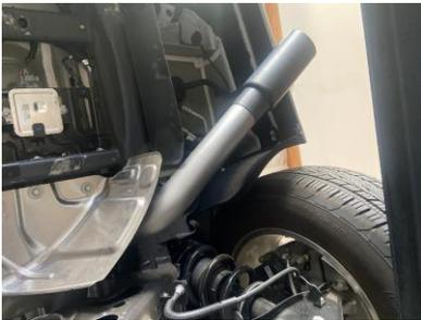
5. Finally, over axle pipe #C can be installed using the Band Clamp #D. Install the Tip to help set the over axle pipe height. (Tighten all clamps working from front to back.)
