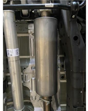
2. TO REMOVE YOUR STOCK EXHAUST, Un Bolt the back half from the flange LOCATED above the rear suspension, then loosen the front clamp and remove the remaining exhaust. **(FACTORY RUBBER HANGER GROMMETS WILL BE RE-USED, USE WD-40 TO AID IN REMOVAL.)**
