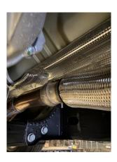
2. TO REMOVE YOUR STOCK EXHAUST, Un Bolt the back half from the flange LOCATED above the rear suspension, then loosen the front clamp and remove the remaining exhaust. (FACTORY RUBBER HANGER GROMMETS WILL BE RE-USED, USE WD-40 TO AID IN REMOVAL.)
