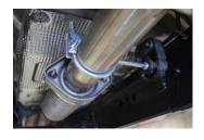
3. Install headpipe #A onto your existing stock 2-bolt flange. Use stock nuts to secure. Do not tighten
