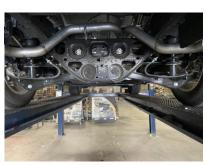
Install the Over Axle Assy. #C into the muffler at least 1-1/2" to 2". #C needs to be installed from the back of the car where the Spare Tire Sits. Use clamp #H to secure pipe to the muffler. Do not tighten. Insert hangers into rubber grommet.
