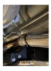
2. TO REMOVE YOUR STOCK EXHAUST, Un Bolt the back half from the flange LOCATED above the rear suspension , then loosen the front clamp and remove the remaining exhaust. (FACTORY RUBBER HANGER GROMMETS WILL BE RE-USED, USE WD-40 TO AID IN REMOVAL.)
