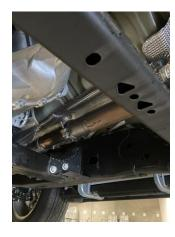
3. INSTALL HEADPIPE #A ONTO STOCK PIPE. INSERT WELDED HANGER INTO RUBBER GROMMET. (You Will be reusing the factory head pipe clamp.)
