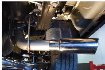
**6.** Lastly, install exit pipe using the last 3" band clamp and adjust according to your desired tip position. Install tip and tighten all bolts and clamps working from the headpipe towards the exit pipe.
