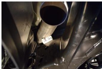
**5.** When installing the overaxle pipe, allow for a 1" clearance between the pipe and the sub-frame.
