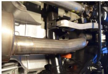
**4.** Install the overaxle pipe into the outlet of the muffler using one of the supplied 3" band clamps.
