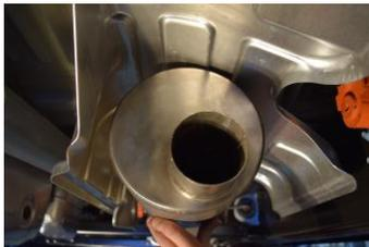
**3.** Next install the muffler by slipping it into the headpipe. Be sure the end marked "Inlet" is installed onto the headpipe. Rotate outlet to 4 o'clock position as seen in picture.
