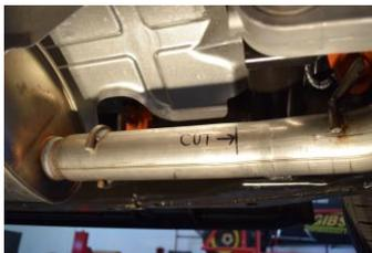
**1.** To remove the factory exhaust, you will need to use sawsall or hacksaw to cut the exhaust at the place indicated in the picture.
