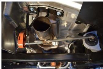
**2.** To install your new Gibson Exhaust, install the supplied headpipe assembly into the factory hangers. Use Bolt Kit.
