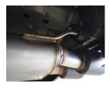
4. Repeat procedure Step 3 to install the passenger side muffler assembly #B.
