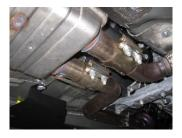
1. To remove your stock exhaust, loosen the two clamps just in front of the resonator and remove the four exhaust hanger brackets behind the rear axle. With the hanger brackets still attached to the exhaust system, remove it from the vehicle.
