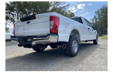
GIBSON EXHAUST systems are designed on a factory stock vehicle. Any aftermarket products installed could increase the sound levels of this Exhaust. Make sure there is a 1" clearance from ALL rubber brake lines, shock boots, fuel lines, tires, etc to prevent heat related damage or fire.
