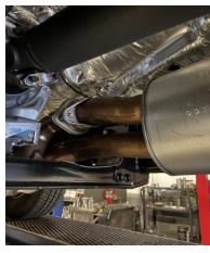
2. TO REMOVE YOUR STOCK EXHAUST, REMOVE IT FROM THE CLAMP LOCATED JUST IN FRONT OF THE RESONATOR. REMOVE HANGERS FROM RUBBER GROMMETS, USE WD-40 TO AID IN REMOVAL, LEAVE GROMMETS IN PLACE.
