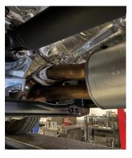
TO REMOVE YOUR STOCK EXHAUST, REMOVE IT FROM THE CLAMP LOCATED JUST IN FRONT OF THE RESONATOR. REMOVE HANGERS FROM RUBBER GROMMETS, USE WD-40 TO AID IN REMOVAL, LEAVE GROMMETS IN PLACE.
