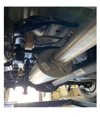
INSTALL MUFFLER # H ONTO HEADPIPE, USE CLAMP #D TO SECURE MUFFLER TO HEADPIPE. DO NOT TIGHTEN. USE A JACK STAND TO HOLD UP THE MUFFLER. OUTLETS SHOULD BE LEVEL.
