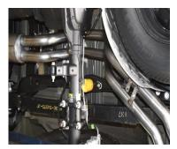
INSTALL PASS. SIDE TAILPIPE #B INTO MUFFLER. INSERT HANGER INTO RUBBER GROMMET, USE CLAMP #E TO SECURE PIPE TO MUFFLER. DO NOT TIGHTEN.
