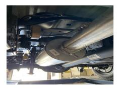
**4.** Install the Muffler #D onto the new Head Pipe using clamp #C. Leave clamps loose enough to have a little play.
