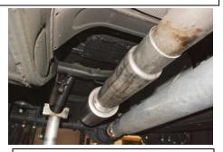
4. Install muffler assembly Item # B onto the head pipe. Use a jack stand to support the muffler while installing the tailpipe. Loosely tighten down the clamp.
