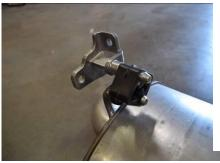
2.Remove the factory exhaust hangers from the using a 13 mm removing the two bolts. These hangers will remain attached to factory muffler when being removed.
