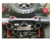
6. Slide the 2.5" band clamp over the expanded part of the muffler and make clamp snug but not tight. Install the Gibson provided tips. Check for exhaust clearance before tightening.
