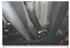
3. Install muffler assembly Item # B onto the head pipe 6". You may need to use a jack stand to support the muffler while installing the tailpipe. Use Item# E to clamp the muffler assembly to the head pipe. Loosely tighten
