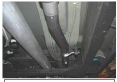
3. Install muffler assembly Item # B onto the head pipe. You may need to use a jack stand to support the muffler while installing the tailpipe. Use Item# E to clamp the muffler assembly to the head pipe. Loosely tighten
