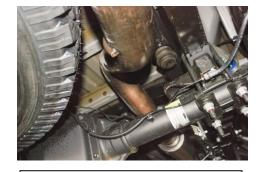
from spare tire install the exhaust tip onto the tailpipe. The system was designed to have the tip 1" below the quarter panel of the vehicle. With the tip in your desired position begin to tighten down all clamp connections from the
