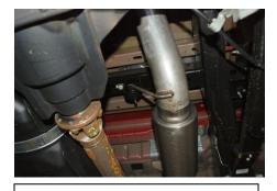
5. Install the over axle pipe. With everything loose you may need to adjust the system for proper clearance of shocks, brake lines, ect.
