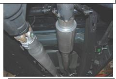
4. Install over axle pipe Item # C into the muffler outlet. Slip the hangers into the rubber grommets and keep tailpipe loose.
