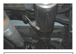
4. Be sure with the muffler supported by the hanger and installed on the head pipes that you keep everything loose to allow for final adjustments.
