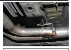
4. Install the Resonator Item #B onto the head pipe Item # A. The inlet of the resonator will have the louvers opening towards the front of the vehicle. Loosely tighten down.
