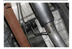
5. Install The muffler assembly Item # C Onto the resonator. Also slide the muffler hanger into the factory rubber grommet. Install the over axle pipe Item # D into the muffler outlet and install the hanger into the rubber grommets. Use clamp Item # F to secure.
