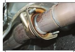
2. Install muffler assembly Item # A into the factory head pipe. Use the clamp Item # E at this connection. Install hanger into rubber grommet and loosely tighten down the clamp.
