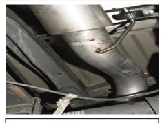
5. With everything loose you may need to adjust the system for proper clearance of shocks, brake lines, ect.
