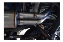
4.NEXT SLIP (#I) 2.5" CLAMP OVER EACH OUTLET OF THE MUFFLER FOLLOWED BY DRIVER SIDE OVER AXLE PIPE. KEEP CLAMPS SLIGHTLY LOOSE FOR ADJUSTMENT.
