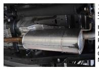
1. FOR AN EASIER REMOVAL OF THE STOCK EXHAUST YOU CAN CUT THE TAILPIPE BEHIND THE MUFFLER USING A HACKSAW. LOOSEN THE FACTORY CLAMP IN FRONT OF THE MUFFLER.NOW REMOVE YOUR STOCK EXHAUST. LEAVE ALL RUBBER GROMMETS IN PLACE. LAY OUT THE EXHAUST AND COMPARE PART NUMBERS.
