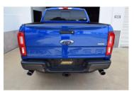
8. INSTALL THE TIPS BY SLIDING THEM OVER EACH EXIT PIPE AND THEN ADJUSTING THEM TO YOUR DESIRED LENGTH AND ROTATION. EXIT PIPES CAN BE ROTATED FOR DESIRE TIP CLEARANCE FROM BUMPER. TIGHTEN ALL CLAMPS STARTING FROM THE FRONT OF THE SYSTEM TO THE BACK.
