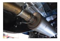
2. SLIDE MUFFLER ONTO THE HEADPIPE 1 <sup>1</sup>/<sub>2</sub>" TO 2". SO THAT THE LOCATOR PIN LOCATES INTO THE NTOCH ON THE MUFFLER ASSEMBLY. USE JACK STAND TO SUPPORT THE MUFFLER. ATTACH CLAMP (#H) AT THE INLET OF THE MUFFLER. DO NOT TIGHTEN.
