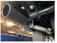
7. INSTALL (J) DRIVER SIDE TAILPIPE HANGER BY SLIDING THE SIDE WITH THE HOLE BETWEEN THE TWO TABS WITH HOLES THAT PROTRUDE FROM THE FRAME JUST ABOVE THE DRIVER SIDE EXIT PIPE LOCATION. NEXT, INSTALL EXIT PIPES USING BAND CLAMPS.
