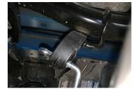
3.INSERT REAR MUFFLER HANGER INTO CORRESPONDING RUBBER GROMMET. THEN YOU MAY SLIDE THE PS OVER-AXLE PIPE (D) INTO THE MUFFLER AND INSERT THE HANGER INTO THE RUBBER GROMMET.
