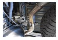
5. NEXT, SLIP 2.5" BAND CLAMP #I OVER THE INLET END OF THE DRIVER SIDE OVER AXLE PIPE (B) AND INSTALL ONTO END OF OVER AXLE PIPE (A) . KEEP CLAMP SLIGHTLY LOOSE FOR ADJUSTMENT
