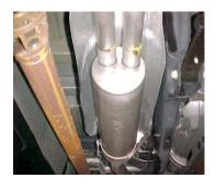
INSTALL MUFFLER # B ONTO HEADPIPE 1 ½" TO 2". USE CLAMP '# G TO SECURE MUFFLER TO HEADPIPE. DO NOT TIGHTEN. USE A JACK STAND TO HOLD UP THE MUFFLER. OUTLETS SHOULD BE LEVEL.
