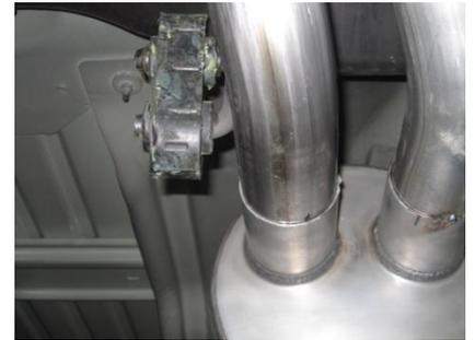
2. Install head pipe #A onto your factory pipe using your stock clamp insert welded hanger into the rubber grommet leave clamp loose.
