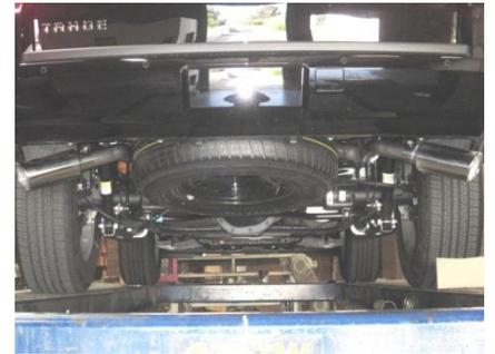
5. Next install drivers side rear hanger and grommet with bolt kit provided. See picture the hanger goes on the outside of the frame and bolts through the first wall of the frame.
