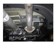
2. To remove your stock exhaust, unbolt the 2-bolt flange located in front of the muffler. Then cut off your tailpipe. Leave all rubber grommets in place. Use WD-40 to aid in the removal of the hangers from the rubber grommets.
