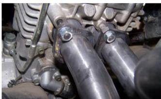
7. To install your Gibson exhaust, first install your header. Re-use the stock nuts to bolt the flanges onto the head. Do not tighten the bolts until the complete system is installed.
