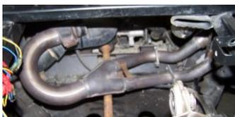
6. Next, unbolt the 2 flanges at the head and remove header. **Do not throw away stock nuts, you will re-use them.** (Lay the stock header sideways in front of sway bar and brake caliper in order to have room to slide the stock muffer out.)
