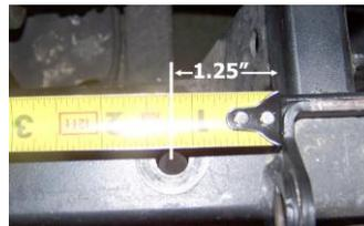
11. Then bolt rear hanger set # D on the top of the factory bed bracket using bolt kit # E
