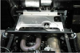
1. Lift and remove bed to access stock exhaust. Remove stock heat shield using a 10mm socket and wrench.
