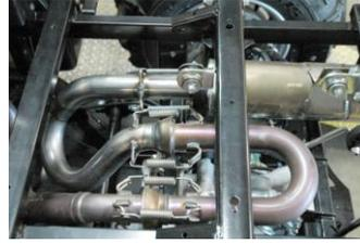
5. After muffler and mid-pipe are in place double check all springs and bolts are in place and tight.
