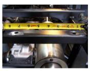
5. Now in the rear frame of your Rhino, you need to drill 2 3/8" holes. The first hole should be 11/4" and the second should be 7 1/8" from the right side of the frame inside of the bed mount bracket
