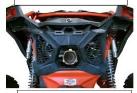
7. Re install the factory exhaust cover. You may need to loosen tip as you install the exhaust to find the right fit. Be sure you have clearance from all components and now drive. After your first ride please double check all clearances and re tighten all components.
