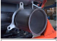
4. Re Install your Factory spark arrestor and tip onto the Gibson Exhaust using the factory hardware. You may need to re adjust the angle once installed on the vehicle with the factory beauty plate.
