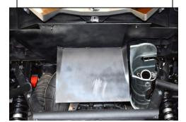
5. Install The Gibson provided under bed heat shield. There are four existing mounting points under the bed. You will loosen the four bolts up install the plate and re install the factory hardware. Check clearance for rattles and tighten down.
