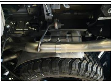
7. Lastly, install exit pipes (F) and tips (L) onto both Driver side and Passenger over-axle pipes. Position the exit pipes to what meets your expectations.
