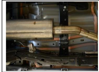
2. Once the factory exhaust is removed, you may begin to install your new Gibson Exhaust. Start with the head pipe using the factory clamp.
