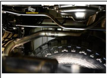
5. Continue by installing Passenger Side passenger over-axle pipe (D). Do not tighten using clamp #H to attach to muffler outlet.
