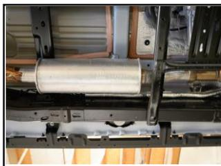
2. To remove the stock exhaust Start by removing the spare tire and the heat shield. Next, cut the exhaust behind the second Muffler. Finally, loosen the clamp securing the headpipe and remove the entire system.
