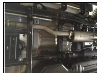
4. Slide the band clamp #E onto each end of the muffler. Next install muffler assembly #B headpipe 1½"-2", with the louvers facing towards the converter. Make sure you slide the muffler hanger into the stock rubber insulator. Use a jack stand to support the muffler. Do not tighten clamp. Muffler inlet is looking into the louvers.
