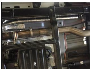
3. Install head pipe # A onto your existing stock front pipe and attach with the factory band clamp. Keep clamp slightly loose.
