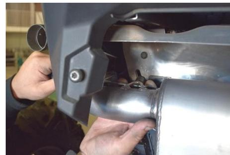
2. Remove the factory exhaust by un-bolting the factory rear shield that covers the muffler. You will re-use the hardware for the Gibson install. Disconnect the 2 factory springs and unbolt the factory exhaust. **Do not damage the factory exhaust gasket.** You will re-use this gasket.
