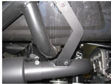
Next install tailpipe brackets onto existing bolt using the 6mm flange nuts provided use some red locktight on these leave loose till install is complete. Next install hardware to bolt the bracket to the tailpipes use red locktight on these also.
