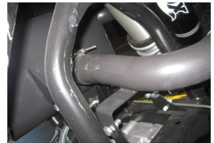
Install the headpipe into muffler make sure you slide the clamp onto the muffler first, use hardware provided to bolt down the headpipe. Next remove the exhaust gasket from the stock muffler and install into you new headpipe. (this is needed to seal the headpipe to header)
