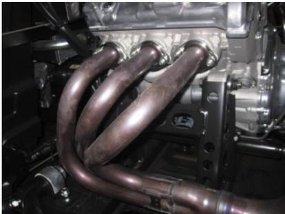
Re install your factory header using the stock hardware make sure to insert it into the new headpipe.
