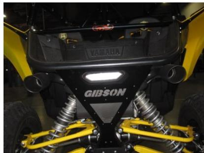
Adjust your kit so the tips are coming out level tighten all nuts, bolts and clamps. Re install rear shock by installing upper bolt first.
