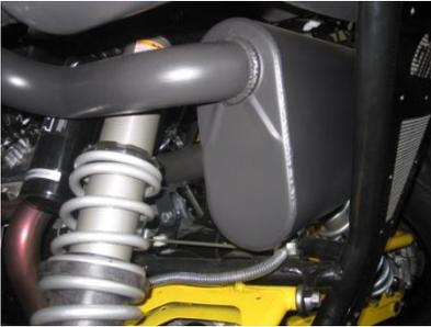
Install your Gibson muffler assembly into the frame using the hardware provided leave all hardware loose til the last step this is important for adjustments in the final step.
