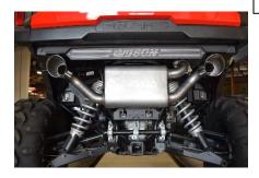
5. Install your new Gibson muffler assembly(Item A) in the reverse order of steps 1 and 2. Use the supplied shorter flange springs(Item E) in place of the factory springs and fully tighten spring bolts.
