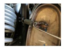
2. Then remove the second retaining spring on the left side of the muffler.
