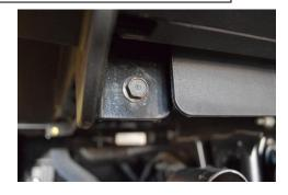
4. Install the supplied beauty plate (Item B) by removing the bolt under the tailgate on each side of the vehicle. Remove one of the screws under the bed that lines up with the bracket on the beauty plate. Then install the beauty plate reusing the same factory hardware.
