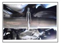
2. Using a jack-stand or muffler stand to support the factory mid-pipe, slide the supplied 3" Clamp (Item D) onto the entrance of the Y-Pipe (Item A) and then slip the Y-Pipe onto the factory mid-pipe. Be sure to locate the notch around the pin in the factory mid-pipe. Keep clamp slightly loose.
