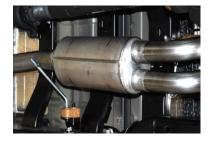
SLIP MUFFLER #B ONTO THE HEADPIPE 1 ½" TO 2". THE OUTLETS WILL BE LEVEL. USE CLAMP #G TO SECURE MUFFLER TO HEADPIPE. DO NOT TIGHTEN.
