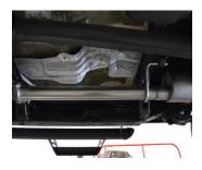
INSTALL HEAD PIPE #A ON TO YOUR EXISTING STOCK 2-BOLT FLANGE AND SECURE WITH BOLT KIT #F. INSERT WELDED HANGER INTO RUBBER GROMMET. DO NOT TIGHTEN
