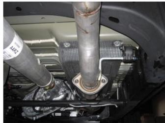
3. Install head pipe #A onto flange. Use your factory nuts.. Insert hanger into rubber grommet. Do not tighten. **\*On short beds cut 12.5" off head pipe**
