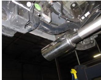
8. Install stainless steel tips. Clamp down. When you have everything in place, firmly tighten all bolts and clamps down securely. Inspect all fasteners after 25-50 miles of operation and re-tighten as necessary.
