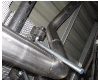
7. Install passenger side tailpipe #D into muffler 1.5-2". Insert welded hanger into rubber grommet. Use clamp #H to secure. Do not tighten. Install exit pipes #E onto tailpipes. Use clamps #H to secure pipes together. Do not tighten. Use zip ties to secure brake and fuel lines away from exhaust.
