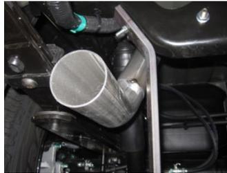
7. Install Spare tire Bracket on drivers side of Spare tire sub-frame as shown in the photo. Spare tire bracket will help keep the spare tire from rubbing on tailpipe. You will remove the factory spare tire heat shield. Be sure after install you have a minimum of 1.5" on all pipes from the spare tire.
