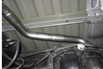
6. Install driver side tailpipe #C into muffler 1.5-2". Rotate until it lines up with the driver's side rear tailpipe hanger #F
