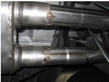
4. Install muffler #B onto headpipe #A 1.5-2". Use a jack stand to support the muffler. Use clamp #f to secure muffler to headpipe. Do not tighten.
