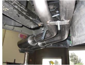
5. Install the driver side over axle tailpipe #C into muffler 1.5-2". Use clamp #G to secure tailpipe and muffler. Insert welded hangers into rubber grommets.
