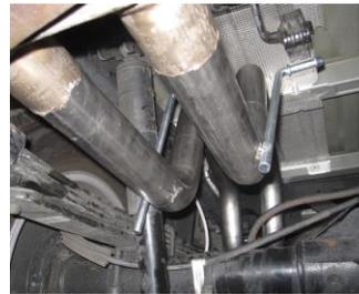
6. Install passenger side tailpipe #D into muffler 1.5-2" and attach with clamp #G. Use bolt kit #H to attach the tailpipes together. Do not tighten. Insert welded hanger into rubber grommet.
