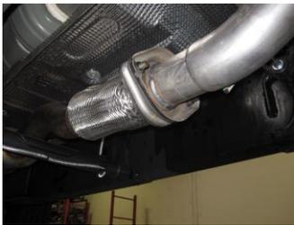
3. Install headpipe #A onto your existing stock 2-bolt flange. Use stock nuts to secure. Do not tighten
