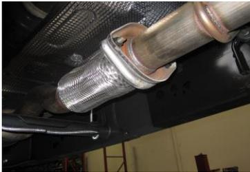
2. To remove your stock exhaust, unbolt the 2-bolt flange located in front of the muffler. For an easier removal of the factory exhaust cut off your tailpipe behind the muffler outlet. Leave all rubber grommets in place. Use WD-40 to aid in the removal of the hangers from the rubber grommets.
