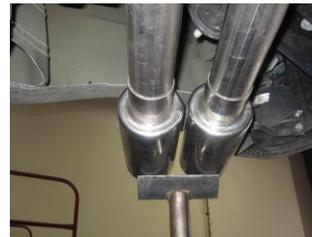
7. Install stainless steel tips. Clamp down. When you have everything in place, firmly tighten all bolts and clamps down securely. Inspect all fasteners after 25-50 miles of operation and re-tighten as necessary.
