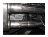
4. Install muffler #B onto headpipe #A 1.5-2". Use a jack stand to support the muffler. Use clamp #f to secure muffler to headpipe. Do not tighten.
