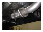
3. Install headpipe #A onto your existing stock 2-bolt flange. Use factory nuts to secure. Leave loose until the whole system is installed. Insert welded hanger into rubber grommet. On short bed cut 12.5" off headpipe.
