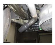
7. Install exit pipe #d onto the tailpipe, use clamp #F to secure the two pipes together. (Rotate for the best fit on your vehicle.)
