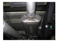
4. Install muffler #B onto headpipe #A 1.5-2" with louvers facing towards the converter. Use a jack stand to support the muffler
