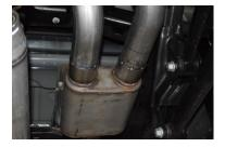
Install head pipe # A Use a jack stand to support the factory exhaust. Do not tighten.
