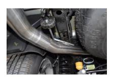
Install the driver side tailpipe # D into the muffler at least 1-1/2" to 2". This pipe will route over the axle and between the Frame rail and tire. Use clamp #J to secure pipe to the muffler. Do not tighten..
