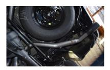
Install exit pipes # E and #F Use clamps #I to secure exit pipes to tailpipes. The system is a universal kit and will require some adjusting to find the optimum position for your vehicle. Sometimes the muffler outlets may need to be rotated slightly to help find the perfect fit.
