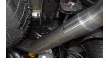
Install the passenger side tailpipe # C into the muffler at least 1-1/2'' to 2". Use clamp #J to secure pipe to muffler. Do not tighten.
