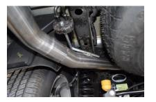
Install the driver side tailpipe # D into the muffler at least  $1-1/2^{n}$ to 2". This pipe will route over the axle and between the Frame rail and tire. Use clamp #J to secure pipe to the muffler. Do not tighten.
