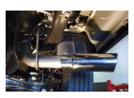
**6.** Lastly, install exit pipe using the last 3" band clamp and adjust according to your desired tip position. Install tip and tighten all bolts and clamps working from the headpipe towards the exit pipe.
