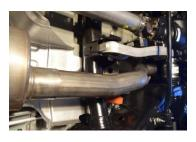
**4.** Install the overaxle pipe into the outlet of the muffler using one of the supplied 3" band clamps.
