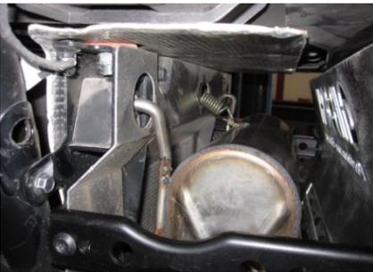
3. Next install the Gibson Muffler assembly. Install the top hanger mounts first then slide the inlet over the factory head pipe reusing the factory nuts to secure flange. Tighten the nuts to factory torque spec.
