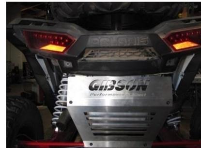
5. Use the factory bolts to install. Once they have been installed tighten the Gibson brackets at the RZR frame. Adjust plate for a level finish. Recheck all hardware for tightness and then go have fun.
