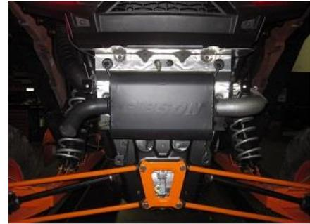
4. Reinstall factory springs on muffler and ensure muffler is positioned correctly in the factory location.
