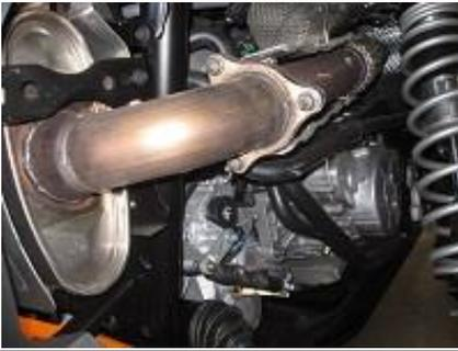
2. Once you have removed the heat shield loosen the factory exhaust. Unbolt the headpipe entirely and remove the factory exhaust.
