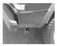
6. INSTALL THE STAINLESS TIP. ROTATE AND SLIDE TIP TO DEISRED LOCATION AND FIT. NOW TIGHTEN ALL CLAMPS, HANGERS, AND BOLTS.
