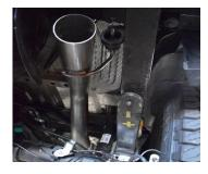
5. SLIDE EXIT PIPE #C USE CLAMP #F TO ATTACH PIPES TOGETHER. ROTATE EXIT PIPE TO ALLOW FOR PROPER CLEARANCE FOR TIP. DO NOT TIGHTEN.
