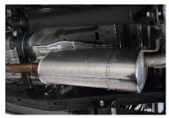
1. LAY OUT THE EXHAUST AND COMPARE PART NUMBERS. FOR AN EASIER REMOVAL OF THE STOCK EXHAUST YOU CAN CUT THE TAILPIPE BEHIND THE MUFFLER USING A HACKSAW. LOOSEN THE FACTORY CLAMP IN FRONT OF THE MUFFLER.NOW REMOVE YOUR STOCK EXHAUST. LEAVE ALL RUBBER GROMMETS IN PLACE.
