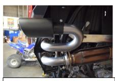
4. Next install the Gibson Muffler assembly. Install the top hanger mounts first then slide the inlet over the factory head pipe re using the factory gasket and bolts. Once in position, install Headpipe and top muffler springs.
