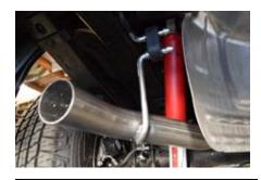
5. Before install of item E, install Driver side hanger bracket(Item G) as shown in picture. Install supplied 2-1/2" band clamp(Item I) onto the inlet side of the driver side over-axle pipe A(Item D) and install onto outlet of muffler. Install hanger into factory rubber grommet hanger. Next install another 2-1/2" band clamp(Item I) onto the inlet side of driver side over-axle pipe B(Item E) and install onto outlet of Item D. Tighten both clamps with allowance for adjustment
