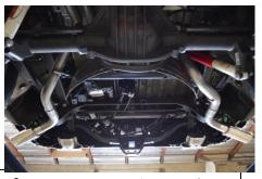
6. Install supplied 2-1/2" band clamp(Item I) onto the inlet side of both the Driver and Passenger side exit pipes(Item F) and install them onto the outlets of each over-axle pipe. Tighten both clamps with allowance for adjustment
