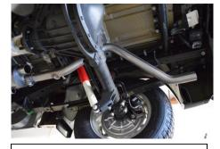
4. Before install of (Item C) install supplied rubber hanger onto factory hanger mount(see picture). Install supplied 2-1/2" band clamp(Item I) onto inlet side of passenger side over-axle pipe(Item C) and install onto outlet of muffler. Install hanger into factory rubber grommet hanger. Tighten with allowance for adjustment.
