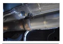
2. Remove clamp from factory head pipe using a small flathead screwdriver to bend up the retaining clip and then install onto new head pipe (Item A).
