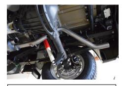
4. Install supplied 2-1/2" band clamp(Item I) onto inlet side of passenger side over-axle pipe(Item C) and install onto outlet of muffler. Install hanger into factory rubber grommet hanger. Tighten with allowance for adjustment
